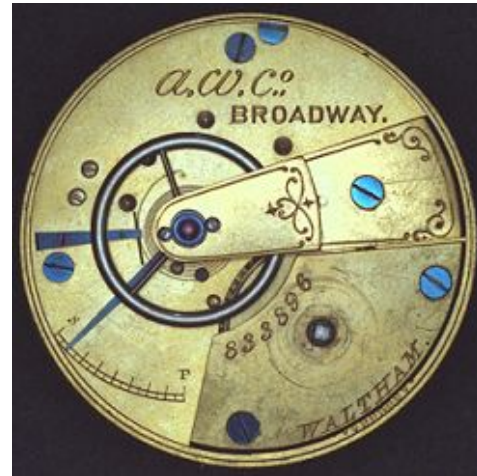
Figure 30. Example Home (715881) and Broadway (833896) Grade Model 57 Movements
