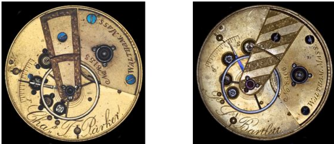
Figure 18. 15J Chas T. Parker 8153 with real jewel settings and 11J P.S. Bartlett 8406 with burnished jewels (Photo of P.S. Bartlett 8406 permission of Hans Dahlke)
